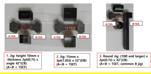
G7000B Welding Jig Base Set can be customized to the user's specifications. (e.g., can change 10mm x 2pt(0.7t) x 42°(CB) set to 10mm x 4pt(1.5t) x 52°(DB) set)
